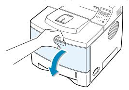
2 Load labels with the print side up. Adjust the guide to fit the width of the labels.
